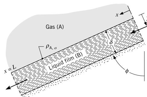
The flow is sustained by gravity, and the gas species A outside the film is absorbed at the liquid–gas interface. The film is in fully developed laminar flow over the entire plate, such that its velocity components in the  $y$  and  $z$  directions are zero. The mass density of A at  $y = 0$  in the liquid is a constant  $\rho_{A,o}$  independent of  $x$ .
