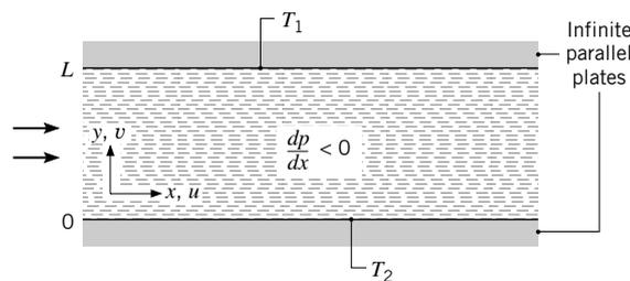
Referred to as *Poiseuille flow* with heat transfer, this special case of parallel flow is one for which the  $x$  velocity component is finite, but the  $y$  and  $z$  components ( $v$  and  $w$ ) are zero.
